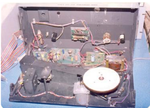
Figure 2: The photograph of gear wheel mechanism of computer based spectrophotometer
