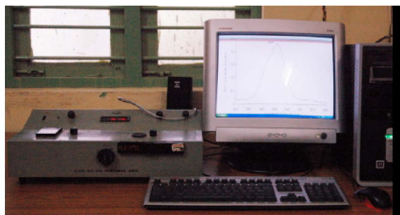
Figure 3: The photograph of complete computer based spectrophotometer
